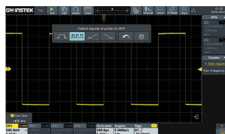
The AUTOSET Button Automatically Identifies Waveforms
